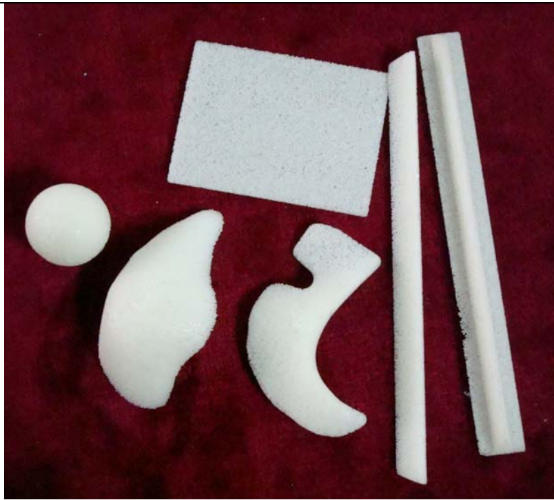
Biocompatible porous polyethylene maxillofacial implants developed at NCL using a unique non-infringing process. The implants have surface and bulk porosity enabling suturing and ingress of tissue.
